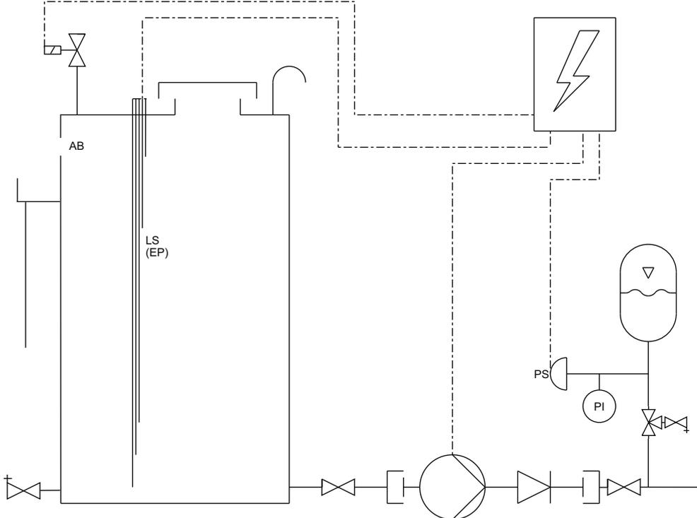
Figure 8: PI&D diagram HUV1 PW with AB overflow
