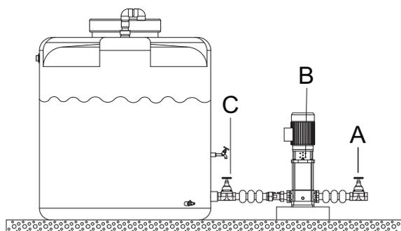
Figure 5: Closed circuit
