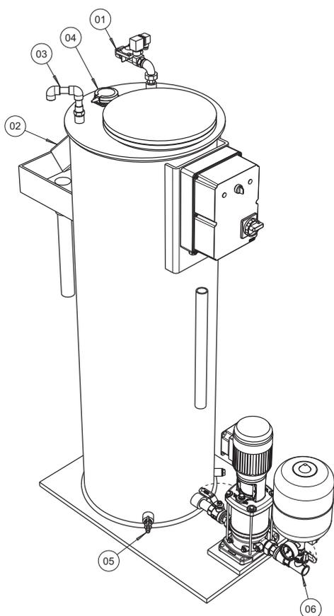
Figure 2: Installations of the type Break-Unit AB break
