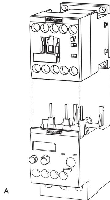
Figure 7: Motor protection relay
